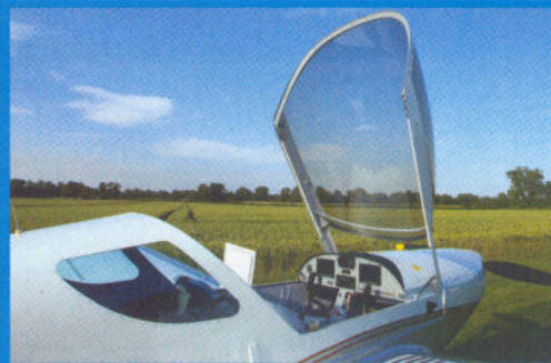
The prototype's tubular steel canopy frame has been changed for one made from composites
