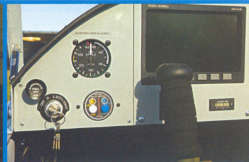
You can vary the propeller pitch in flight: yellow for finer, bleue (Zidane?) for coarser
