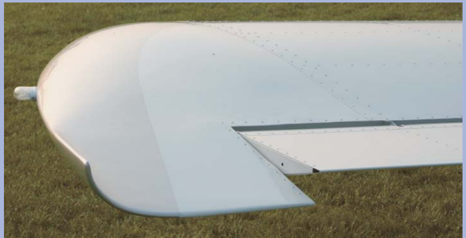
Wings (above), fin, rudder, tailplane and elevator all feature high quality composite tips.
