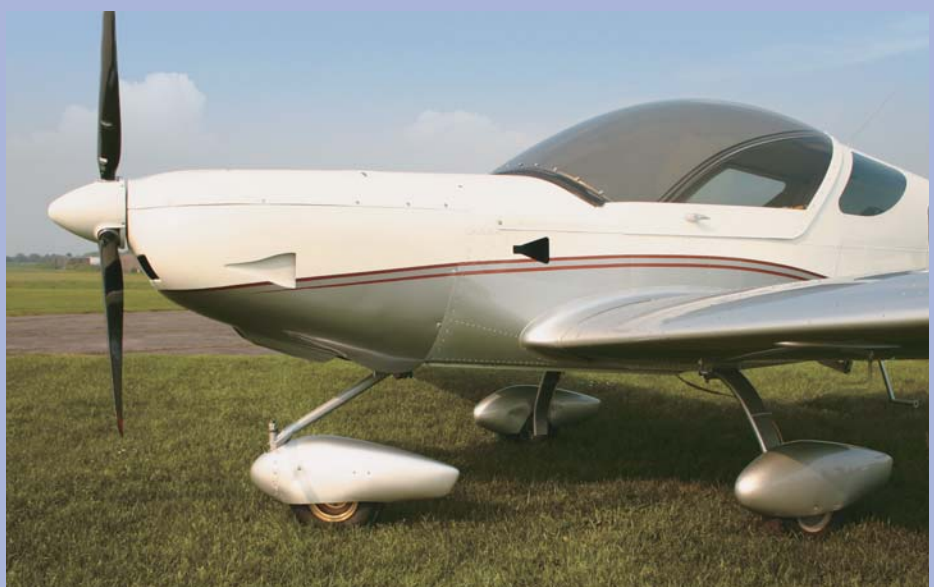
Main gear is via undamped twin composite legs, and steel nose gear features rubber in compression and castoring nose wheel. Note also the handy step just behind the wing trailing edge.
