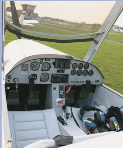
This general cockpit shot highlights the overall high quality of the interior finishing. Production kits will feature a narrower centre console and more forward placed throttle quadrant to enable stronger, wider seats to be fitted.
