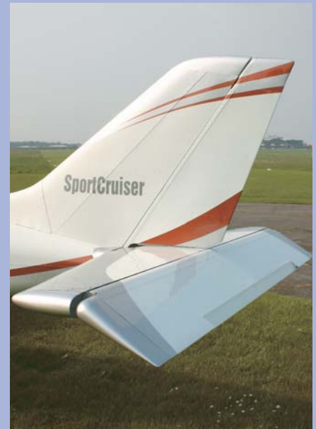
Swept fin and rudder give the Sport Cruiser a graceful look. Note large, electrically operated trim tab.
