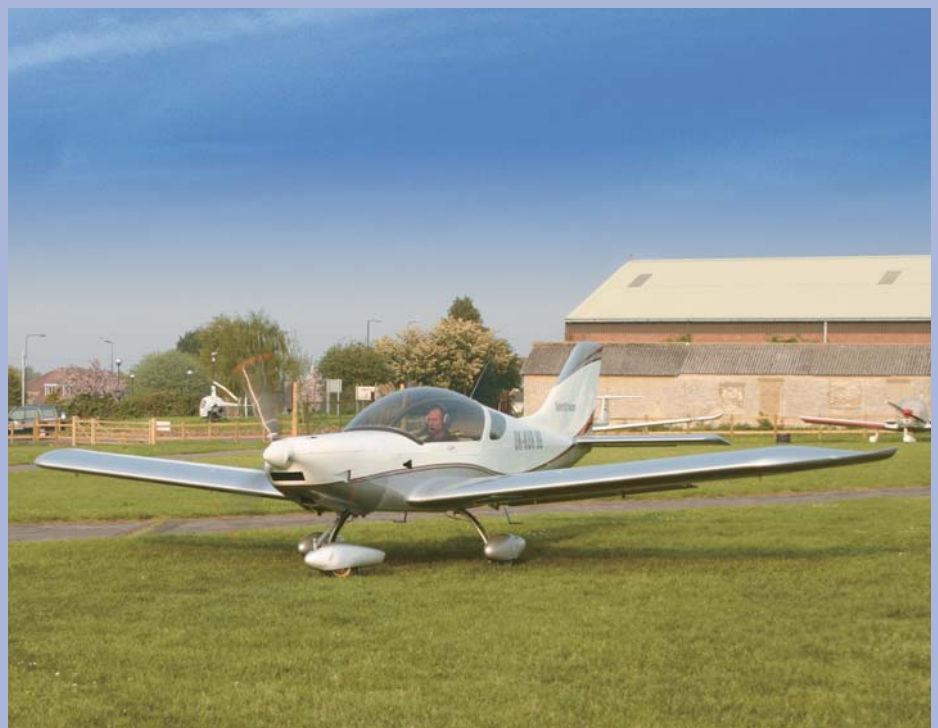
Wings (above), fin, rudder, tailplane and elevator all feature high quality composite tips.
