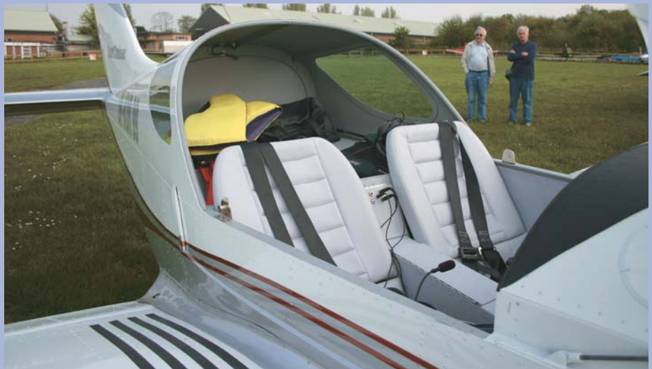
Ample behind the seats baggage area compliments the wing lockers. Note also the full upper torso harnesses. The external channelling under the top longeron houses the optional ballistic parachute's cable. This will be moved into the new, composite canopy frame on production models. The actual chute is housed under the starboard side coaming.
