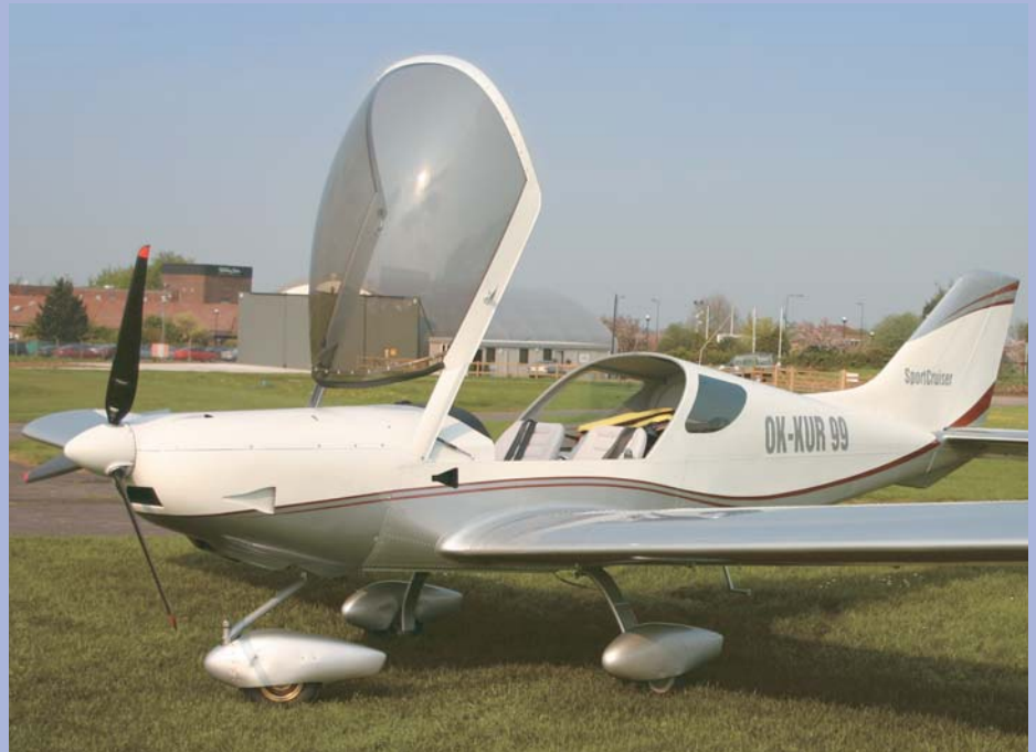
The large, forward hinged canopy is supported by a gas strut, which alleviates the need for Schwartzenegar sized arms. Closure is via two automatically catching, car type latches.
