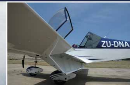
Large efficient flaps significantly enhance teamEurostar performance.
