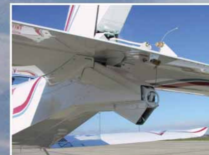
Optional towing equipment for efficient glider and banner towing.
